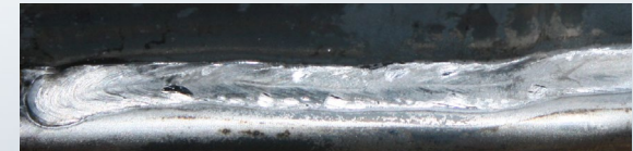
Weld seam after cleaning
